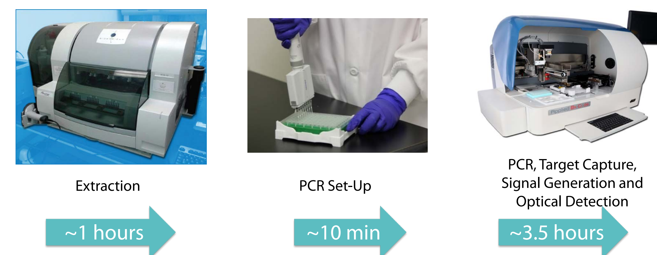
Figure 2. Workflow for BioCode® RPP (top) and schematic for BioCode® MDx 3000 deck layout (bottom). 192 samples in an 8 hour shift with minimal hands on time. This system is designed to run 3 different BioCode® panels simultaneously in one run.
