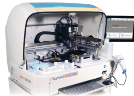
STEP 3: Load PCR microplate onto BioCode® MDx-3000. The System automates the PCR amplification, hybridization/target capture, and detection process, and reports the results.
